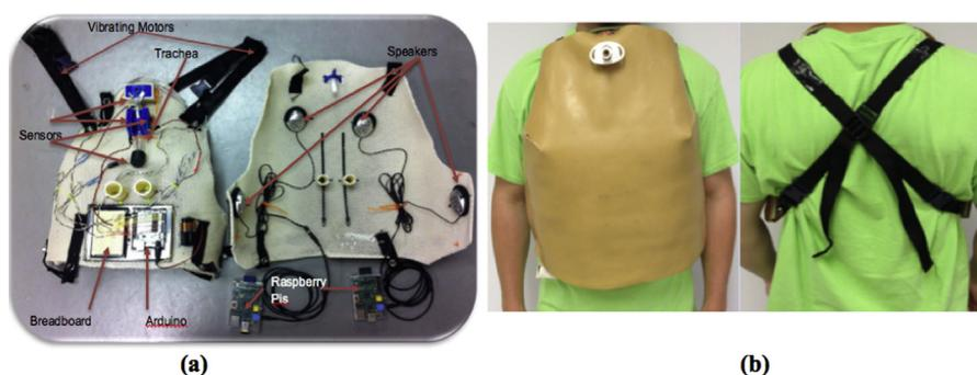
**Figure 1** The Tracheostomy Care Overlay System, showing (A) Interior components and (B) anterior and posterior views of the device being worn by a live actor.
